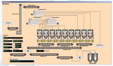
**KSA** is a modular system for the manual and automatic control of the processes in the gravel plant. It consists of the administration software **KSA-DV** and the plant visualisation **KSA-VISU**. Thanks to its modular structure, **KSA** allows to create a plant control which is tailored to your specific needs. For this, only the hardware and software modules necessary for your production process will be compiled.
